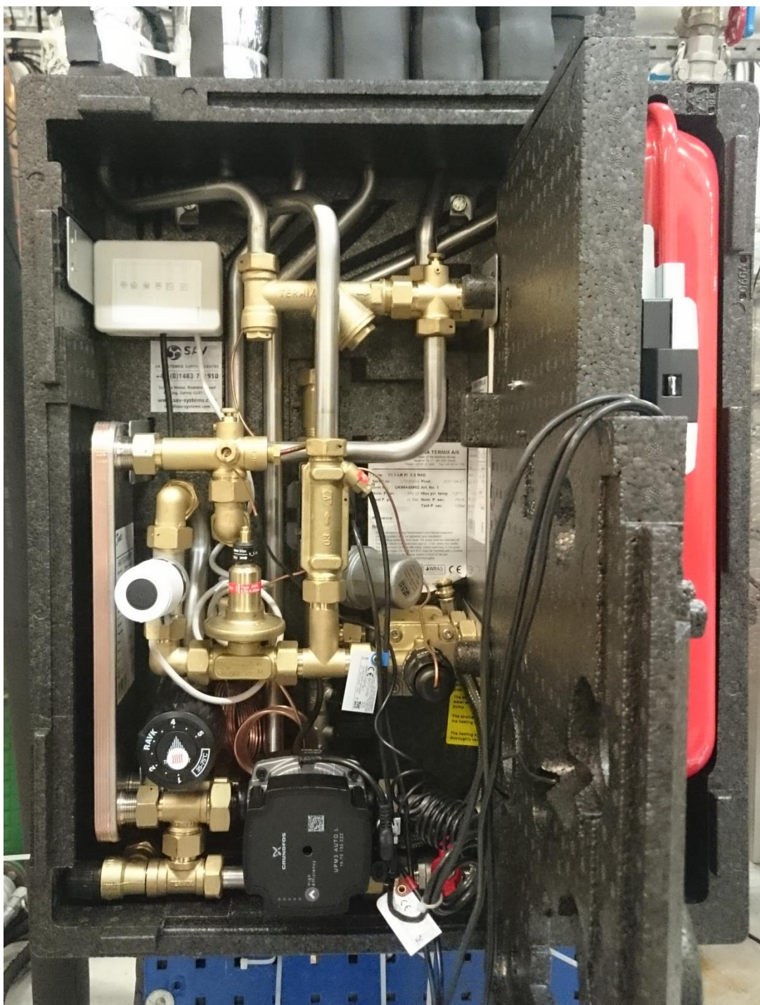
Figure 1. The test object after testing. Insulation removed.
